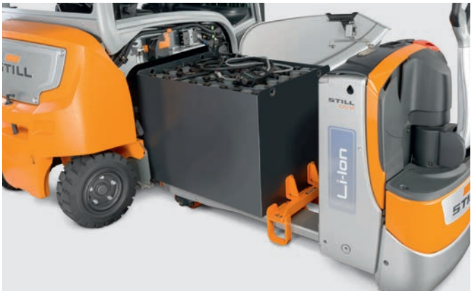
Battery change with electric pallet truck
