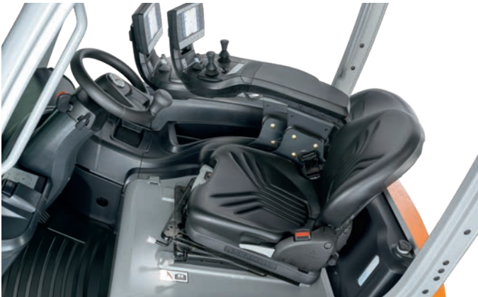
Swivel seat for comfortable reversing
