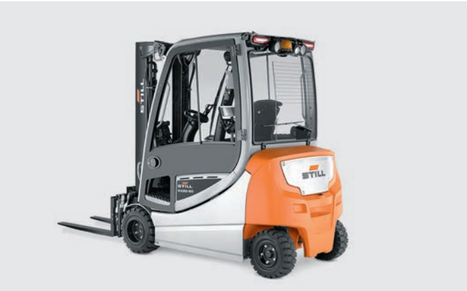
Four-wheel version with fully enclosed driver's cabin for outdoor use
