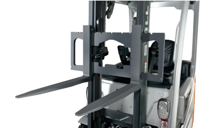
Optimal view of fork tips when loading HGVs
