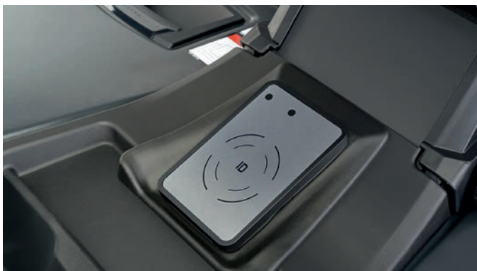
A variety of access control options: optional access via FleetManager or PIN code and standard access via key switch
