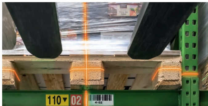
Optional cross line laser for safely aligning the centre of the pallet
