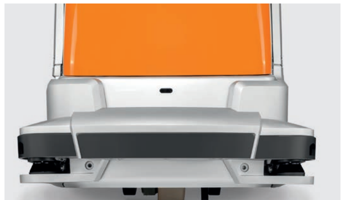
360° pedestrian protection provided by integrated safety laser scanners in the LTX 50 iGo systems
