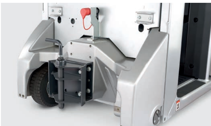
Flexible applications thanks to various connection options for tugger train elements and trailers 2
