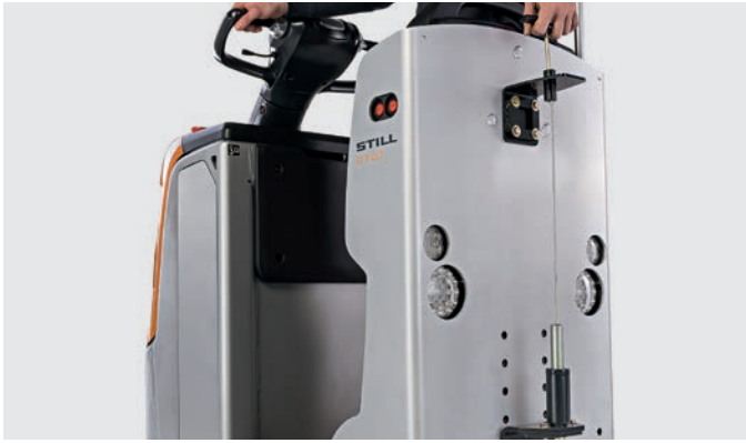
Fast release of coupling from driver's seat 1
