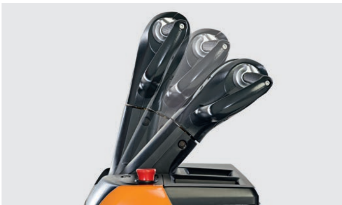
Height-adjustable steering for different operators 1
