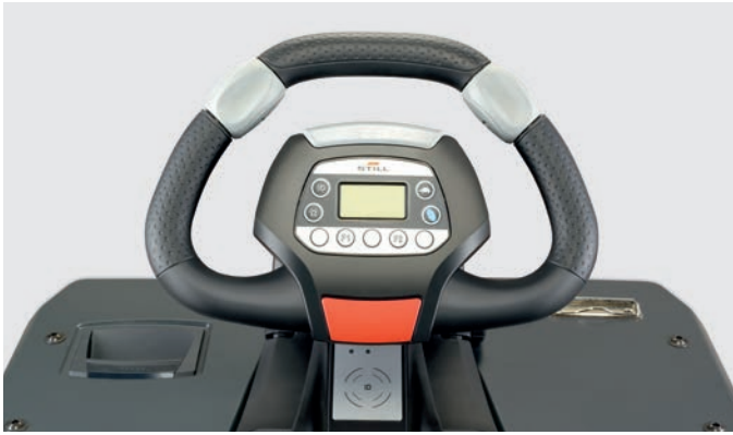
Unique STILL Easy Drive steering wheel for optimised driver control and operation of all functions without changing grip 2
