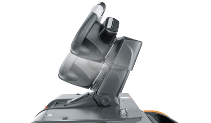
Optimal adaptation to individual operator preferences thanks to the height-adjustable steering wheel 2
