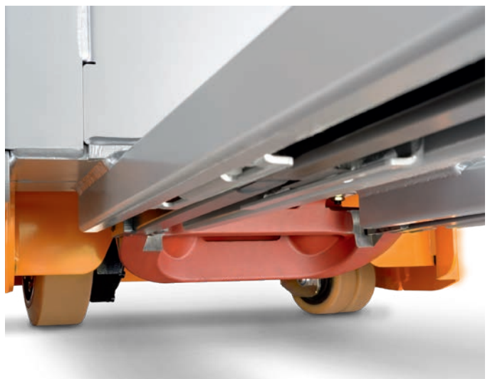
Optional automatic level compensation for uneven floors and best possible handling
