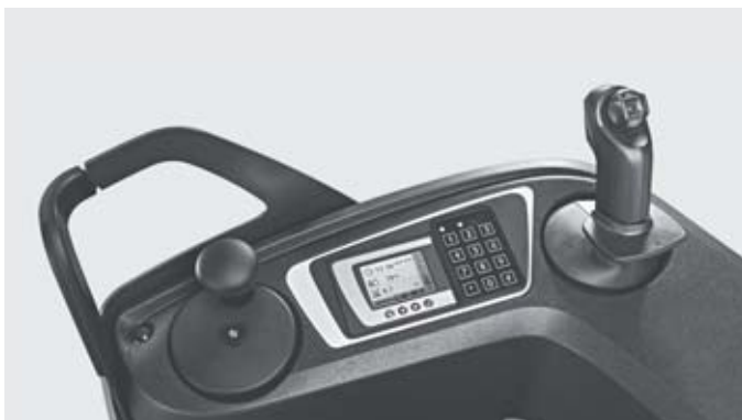
The steering wheel can optionally be positioned on the left- or right-hand side for individual adjustments
