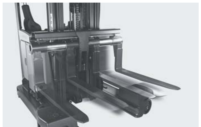
Hydraulic fork-spreading system ensures safe load handling
