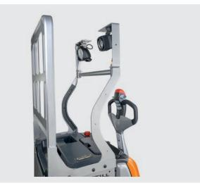
Maximum safety when loading and unloading lorries thanks to STILL Safety Light and working lights
