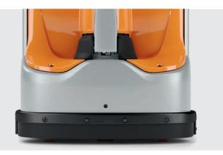
Unharmed feet guaranteed: the active foot stop halts and reverses the truck automatically upon contact with feet  $% \left( {{{\rm{s}}_{\rm{s}}}} \right)$
