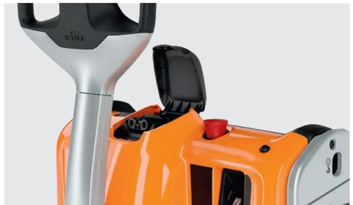
The optional quick-charge access for lithium-ion batteries makes charging even quicker and easier
