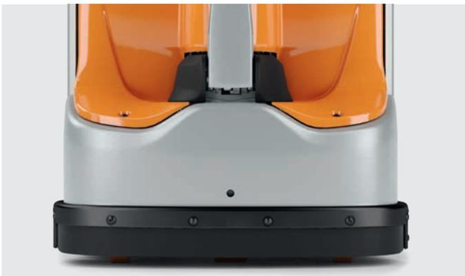
Unharmd feet guaranteed: the active foot stop halts and reverses the truck automatically upon contact with feet
