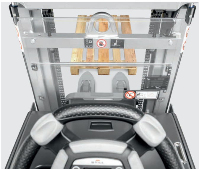
High handling performance and excellent visibility of the load thanks to the free view mast
