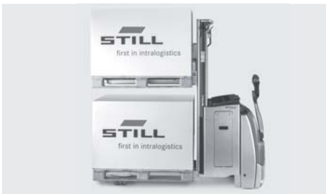
High handling capacity due to simultaneous transport of two non-stackable carriers
