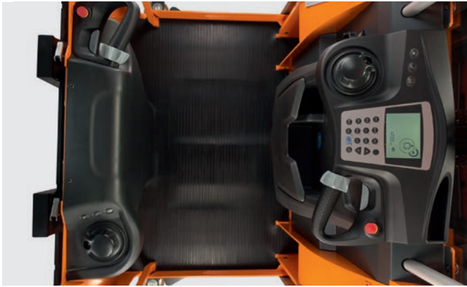
Efficient truck utilisation thanks to optional two-sided operation
