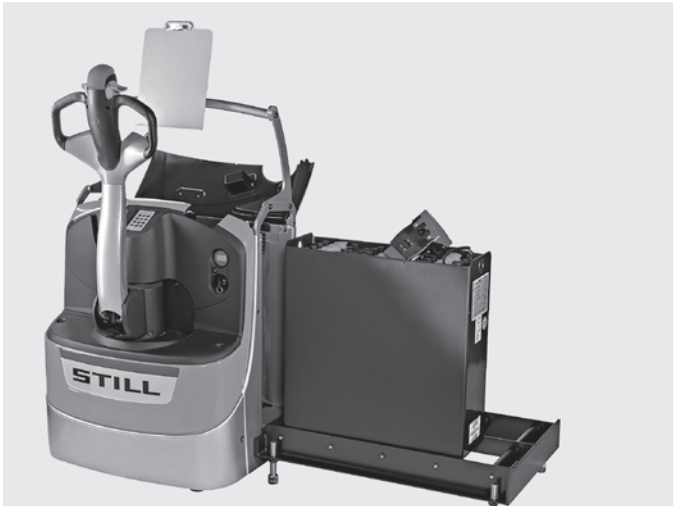
Maximum availability due to lateral battery change
