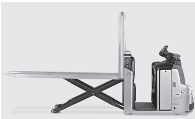
The right level: freely adjustable lifting heights on the OPX-L 20 S iGo neo variant for additional ergonomics
