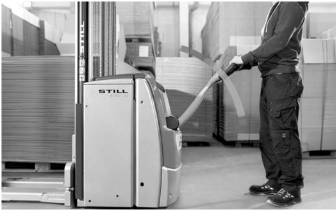
Safety in production: depending on tiller angle, speed is automatically adapted to the distance between the operator and the truck
