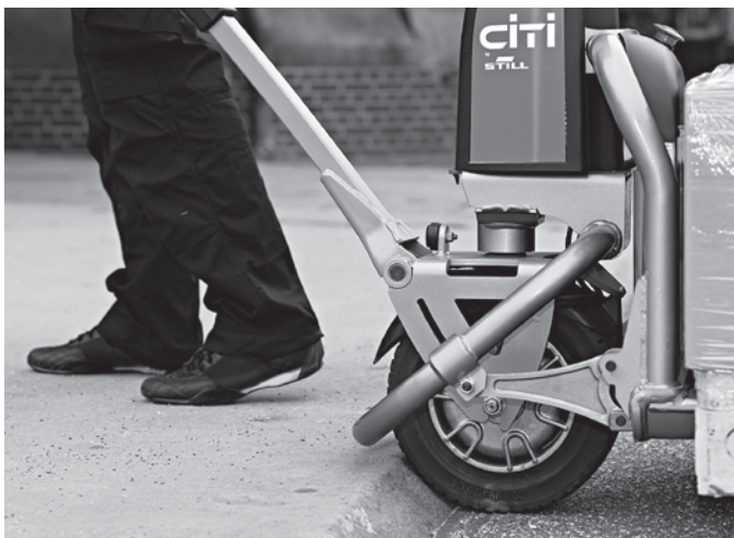
Can be used on any flooring thanks to profiled solid rubber drive wheel 1
