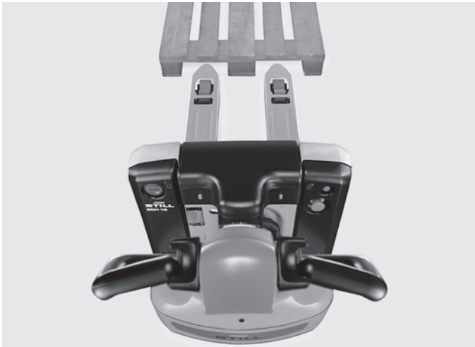
The low height of the pallet truck makes the fork tips easy to see 3
